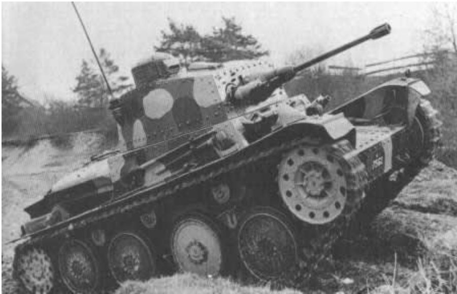
The Czech Panzer 38, eventually uparmored to 50mm frontal and 30mm sides; 37.2mm gun/90 rounds. http://www.wiivehicles.com/germany/foreign/pzkpww_38t.html 9 tons.
